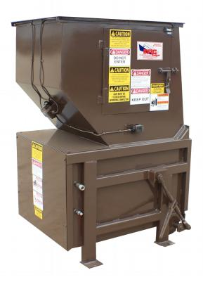
This heavy duty compactor assembly is much stronger than others on the market. 3/16" side walls are reinforced with 1/4" thick structural tube framework and the packing ram face and compaction floor are 3/8" thick plate backed by structural steel channels and 3/8" thick contour shaped ribs. This extra rugged construction provides much longer service life even under extreme conditions.
