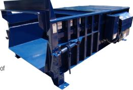
The RJ-275 is stress-engineered for durability. This means the strength is where it belongs– like the half-inch charge box floor reinforced with five heavy-duty steel channels, the half-inch plate ram face backed with 10-inch (254mm) plus 6-inch (152mm) structural channels, and the extra rugged reinforced sides.
